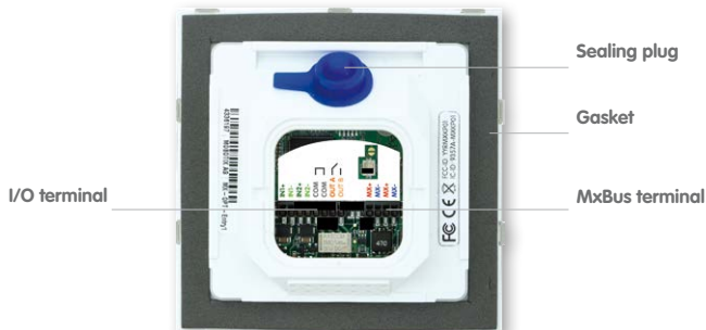
View with housing cover removed
