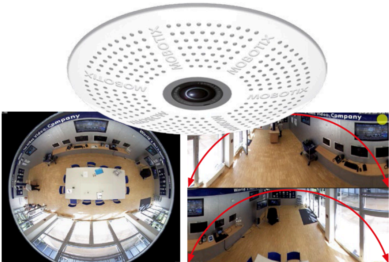
The ceiling-mounted c25 delivers two 180° panorama images of a room.
